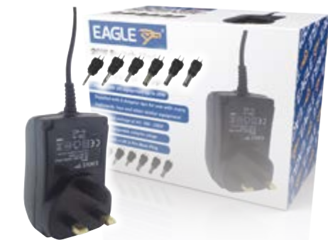
P003EA 24 V DC 750 mA Regulated Switch Mode Power Supply 18W UK Plug • Powers 24V DC equipment up to 20W • Supplied with 6 Adaptor tips for use with many keyboards, toys and other similar equipment. • Wide input voltage of AC 100 - 230V • Fitted with a UK 3-Pin Main Plug
