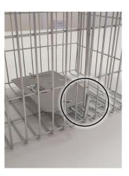
6. The trap is now armed, carefully place bait near the trigger plate and place the trap in the required location. Check trap regularly.
