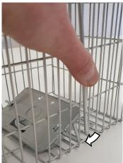
5. Position the trigger rod behind the upright rod of the trigger plate and allow the tension from the trigger rod to hold it in place.
