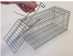
3. Hold the trap door arm down and rotate the locking pin to also lie flat on the top of the trap
