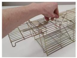
5. While holding the locking pin in place, slide the hoop of the trigger pin over the locking pin
