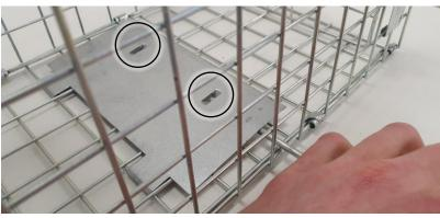
Pull the hook end of the trigger rod up to the hook end of the locking rod
