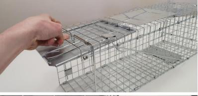
20. Holding the door up, locate the locking pin and move this under the notch on the door
