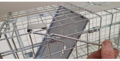
18. To set the trap, push the spring arm inwards and lift the door
