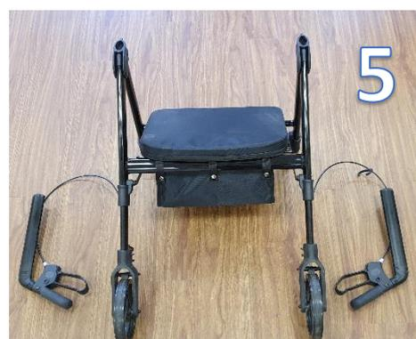
5. Insert the handle assemblies into the uppermost tubes until the locking pins click in place, in the same manner as the legs (Figure 6). *Note: ensure the brake cable lies on the **outside** of the frame, this will reduce the risk of interference or entrapment.*
