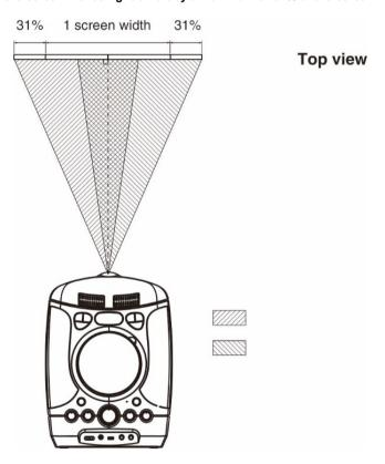
: Picture position when moving the picture to the left at maximum.
