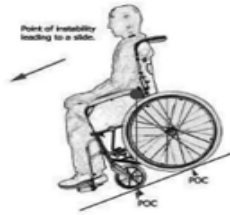
Figure 4 Beginning of instability (slope too steep)
