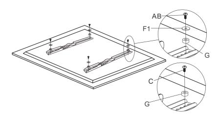
If the television has a curved back or includes an obstruction that may prevent the brackets from fitting flush to the back you can place the spacers beneath the brackets to lift away from the back. The brackets can now be secured with screws A, B or C with the Washer (F1) if necessary.
