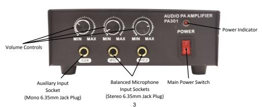
The unit has 2 balanced microphone and 1 auxiliary input. Before switching the unit on turn all volume controls to the minimum position (anti-clockwise) and insert the required microphone or auxiliary equipment. With the volume controls still at the minimum turn the unit on and the power indicator light should illuminate. Turn on the auxiliary equipment or gently speak into the microphone while turning up the required volume control till the desired output level is achieved.
